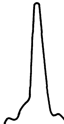
AMPLITUDE MODULATION = ABOUT 50% CAUSING DISTORTION. FREQUENCY MODULATION = 1 MC PER USEC.
